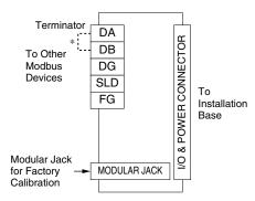
\*Attach the terminating resistor when the module is at the termination of a transmission line.
