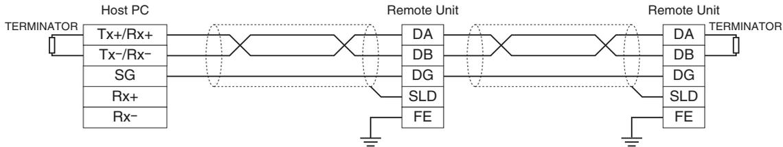
Be sure to connect the terminating resistor across DA and DB at both ends of communication line.
