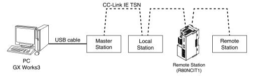
1) Master station, Local Station and Remote Station (R30NCIT1) are connected by Ethernet cable. CN1 and CN2 of CC-Link IE TSN Network RJ-45 modular jacks can be connected in any order.
