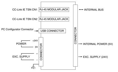
Regarding CN1 and CN2 of RJ-45 connector for CC-Link IE TSN network, there is no restriction for connection order
