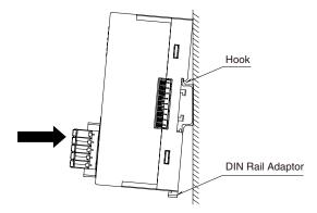
Position the upper hook at the rear on the DIN rail and push in the lower. When removing the module, push down the DIN rail adaptor utilizing a flat-blade screwdriver and pull.
