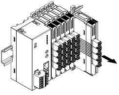
• Removing an intermediate module
