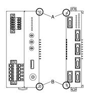
Confirm that the locking clamps of the I/O module are set. Insert the module in parallel to the next one while aligning the grooves of both modules (A & B in the above figure). Maintain it perpendicularly to the rail.
