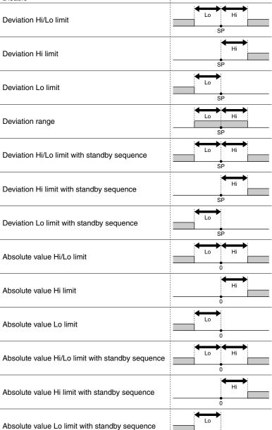
Standby sequence is a function to prevent unwanted alarm triggered at the startup or at an SP change. If the PV is in alarm range at the startup or at an SP change, no alarm is triggered until the PV is out of the range. Once it is out and then in the range again, normal alarm function starts functioning.
