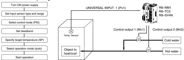
Note: The examples above are for single loop, however, dual loop control is also available using only one R8-TC2.
