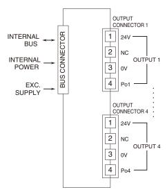
Note: Pin 1 of output connector is connected to 24V of the excitation supply. Pin 3 of output connector is connected to 0V of the excitation supply.
