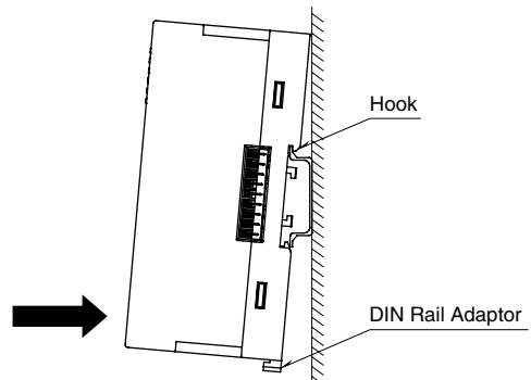
Hang the upper hook at the rear on the DIN rail and push in the lower. When removing the module, push down the DIN rail adaptor utilizing a minus screwdriver and pull.
