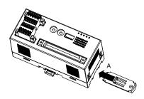
B)Set the upper hook at the rear side of the unit on the DIN rail.
