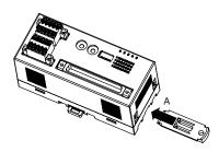
B)Set the upper hook at the rear side of the unit on the DIN rail.
