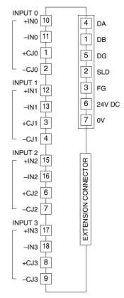
In order to improve EMC performance, bond the FG terminal to ground. Caution: FG terminal is NOT a protective conductor terminal.
