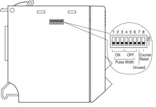
Note: Counter Reset SW is normally OFF during operation.
