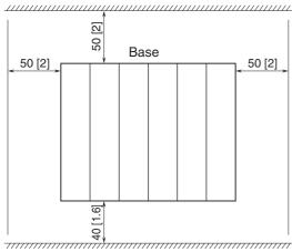
Panel bottom or wiring conduit (height ≤ 50 mm or 2 in.)
