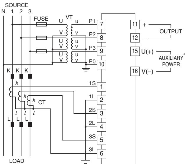
\*The transducer can be powered from the input voltage when the voltage is sufficiently stable and meets within the range of auxiliary power supply of the unit specified in the data sheet/instruction manual.
