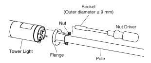
• M17 nuts for the L-shaped bracket are temporarily locked. Re-tighten them firmly after adjusting the position. (Torque:  $24 - 26 \text{ N} \cdot \text{m}$ )
