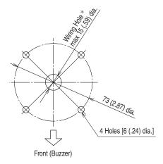
\* Protect wires to prevent scratching them on edges. Determine the hole diameter according to the size of the wires.
