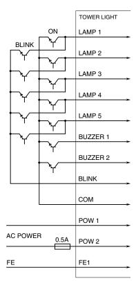
Note 1: Do not set lamp ON input to "On" and BLINK input to "Blink" at the same time watsoever, it might result in shortcircuit. Note 2: In order to improve EMC performance, bond the FE1 terminal to ground.
