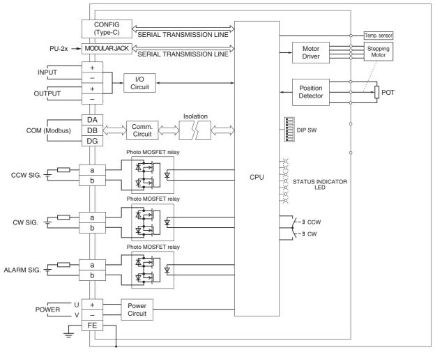
Note1: No polarity between a and b.
