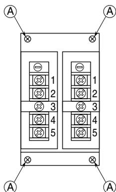
Mounting screws with washer for attaching power unit, M3 x 5 screws, 2 pls. per unit
