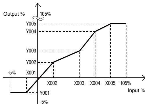
When the input to be converted does not match any X value in the table, two X values which are closest to the input in positive and negative directions are selected and linearly interpolated, thereby obtaining a Y value to be outputted.
