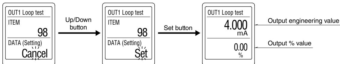
Note: While the loop test is performed, all input signals are disregarded.
