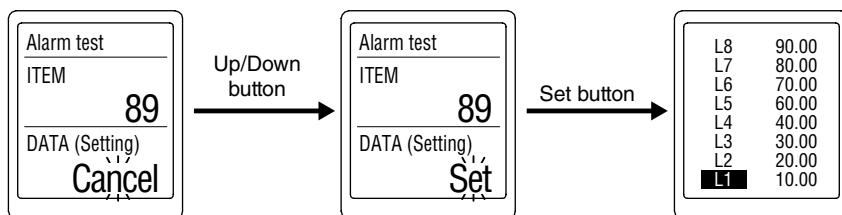
\*<sup>1</sup>. While alarm test is being performed, actual input is disregarded.
