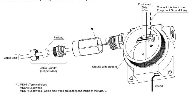
\*2. For wiring the MD6T, a cable gland is required. The packing of the cable gland must be separate from the body. Choose an appropriate one for the environment in which the surge protector is used.
