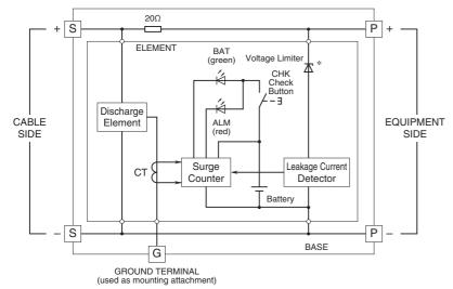
\* The zenor diode has polarity. Zero-cross signal cannot be connected.
