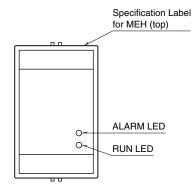
The MEH's model suffix codes change according to the power input voltage. Check the specification on the label.
