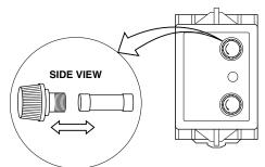
In order to remove the fuse, turn it counterclockwise and pull it out of its holder.
