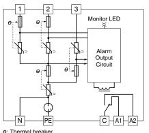
Note: Terminals C, A1 & A2 are available for 'Alarm output' code 'A.' The schematic shows the relay contact status of a thermal trip or power off.
