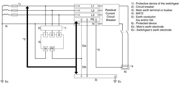
\*1. The circuit breaker must be installed.
