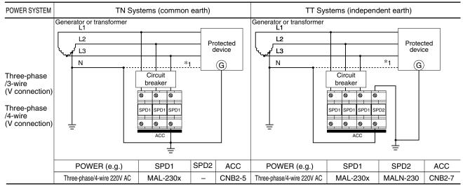
\*1. Wiring only for three-phase/4-wire
