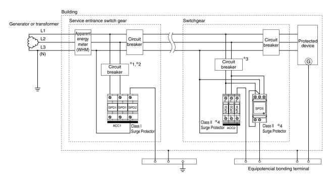
\*1. The circuit breaker's rating current must be of 150 A, and the rated interrupting capacity selected must be the grater between 30 kA or the highest amount of current that could be available in the circuit. For monitoring the operation of the circuit breaker we recommend also using the alarm switch (AL).
