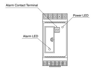
The MDW5ALW consists of a head element and base. The head element incorporates surge suppression circuit, life monitoring circuit and a battery for memorizing the life. The base incorporates power circuit and a relay for alarm output. When the surge suppression circuit is damaged or the battery is weakened, replace the head element to recover the surge protector's performance. Replacing the head element does not disturb the communication.
