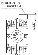
Input shunt resistor attached for current input.
