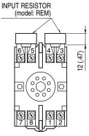
Input shunt resistor attached for current input.
