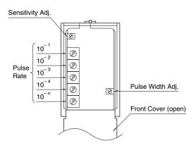
Positions for the rotary switches  $10^{-1}$  through  $10^{-n}$  apply respectively to each digit of the decimals and exponential as shown below.
