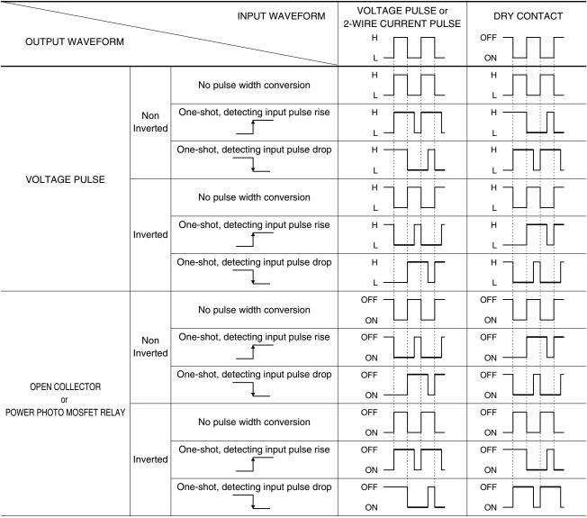
The pulse width in one-shot means the bold lined section of a pulse waveform.
