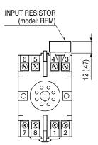
Input shunt resistor attached for current input.
