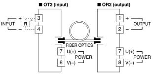
\*Input shunt resistor attached for current input.
