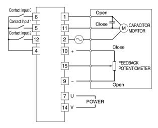
Note: Note that when limit switches inserted in motor wiring, the making/breaking may cause stress on the SSRs.
