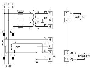
\*CT Protector (model: CTM) attached to these terminals. \*\*The transducer can be powered from the input voltage when the voltage is sufficiently stable and meets other supply voltage requirements.
