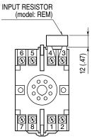
Input shunt resistor attached for current input.
