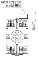
Input shunt resistor attached for current input.
