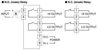
\*Input shunt resistor attached for current input.
