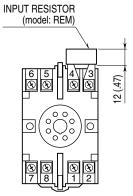
Input shunt resistor attached for current input.
