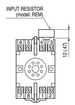
Input shunt resistor attached for current input.
