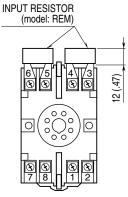
Input shunt resistor attached for current input.
