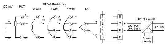
\*1. Short across the terminals 1 & 2 for a resistance or RTD input with 2- or 3-wire connection.
