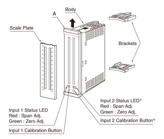
Pull up the part 'A' when replacing the scale plate. \*Not provided for the 48NV-1.
