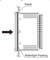
2) Push the mounting brackets into the grooves on top and bottom of the rear module, until they hit the panel's rear side. Leave at least 3 centimeters both above and below the unit for ventilation.
