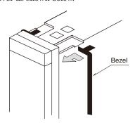
When multiple units are to be clustered side by side, insert one bezel between two units as shown below.
