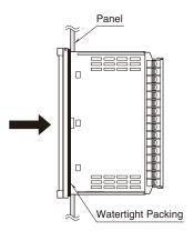
2) Push the mounting brackets into the grooves on top and bottom of the rear module, until they hit the panel's rear side.
