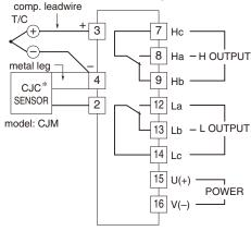
\*Deleted with B thermocouple
