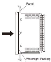
Push the mounting brackets into the grooves on top and bottom of the rear module, until they hit the panel's rear side.
