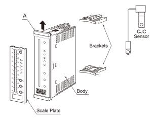
Pull up the part 'A' when replacing the scale plate.
