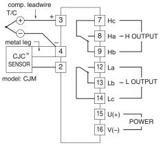
\* Deleted with B thermocouple
