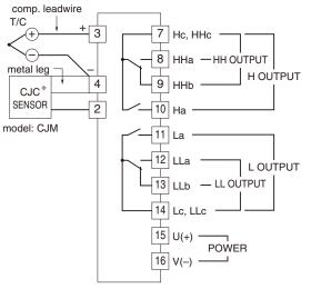
\* Deleted with B thermocouple
