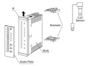
Pull up the part 'A' when replacing the scale plate.
