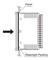
2) Push the mounting brackets into the grooves on top and bottom of the rear module, until they hit the panel's rear
