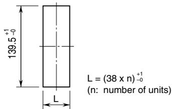
Note 1. A bezel is required between units for high-density mounting.
