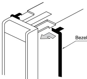
• When installing the meter into a panel, first remove the nameplates at the top and bottom of the front panel. Turn the screws behind these nameplates clockwise until the retaining clips come up and are fixed.
