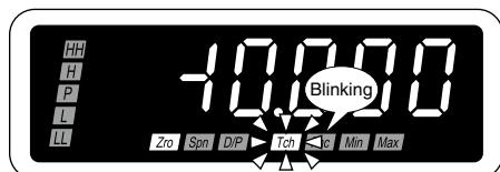
**4** Apply 0% input and press Up button to register the value.
