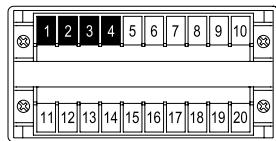
Connect DC voltage or current signal wires. Be careful that the input terminal assignment depends on the input code and type.
