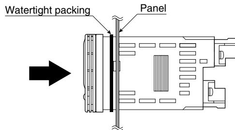
(6) Push the mounting brackets into the grooves on both sides of the rear module, until they hit the panel's rear side.
