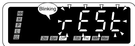
4 Press Alarm/↓ or Scale/↑ button to execute the initialization.
