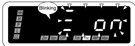
4 Press Alarm/↓ or Scale/↑ button to apply the new setting.
