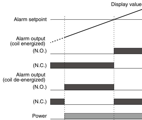
In order to provide an alarm output at power OFF and at alarm, set "coil de-energized" and use the N.C. terminal.
