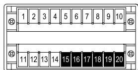
Two or four alarm contacts are output depending on the specified alarm output code.
