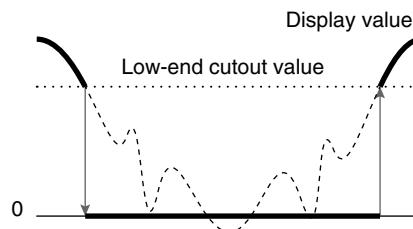
Fluctuation near 0 and negative reading can be cut to 0.
