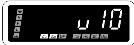
**2** Press Alarm/↓ or Scale/↑ button to go to the analog output function mode setting.
