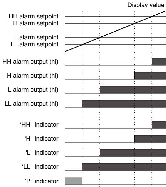
Low or high trip action can be set for each alarm output.
