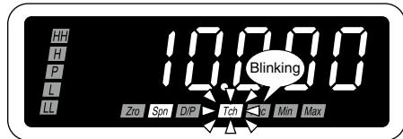
**7** Apply 100% input and press Up button to register the value.
