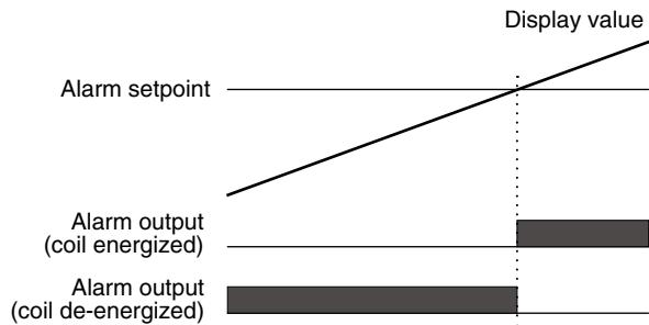
In order to stop operation of equipment when the display value exceeds the setpoint, for instance, set reversal output logic (N.C.), "coil de-energized".
