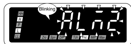
3 Press Alarm/\downarrow or Scale/\uparrow button to apply the new setting.
