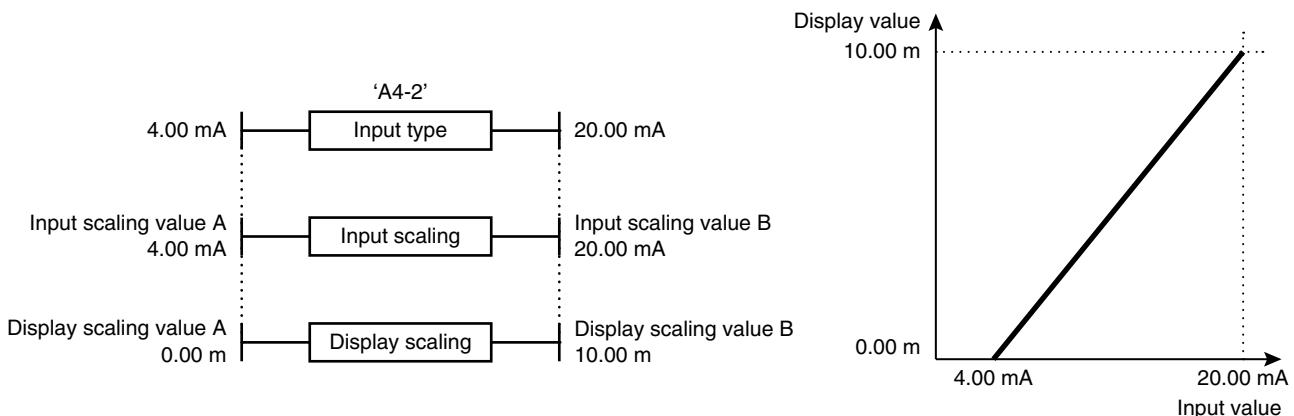
Input type: type of input signal to 47LV (measuring range)
