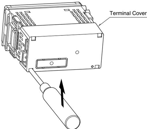
**How to remove the terminal block**
