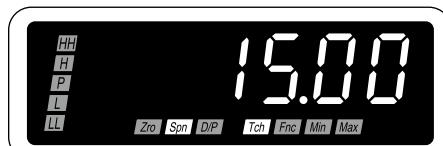
**4** Press Up button to go to the teach calibration (SPAN) setting.
