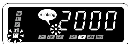
**4** Press Shift and Up buttons to set the LL (L, H or HH) alarm setpoint.
