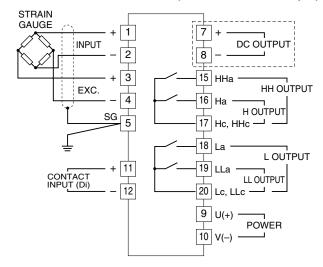
Note: The section enclosed by broken line is only with DC output option.
