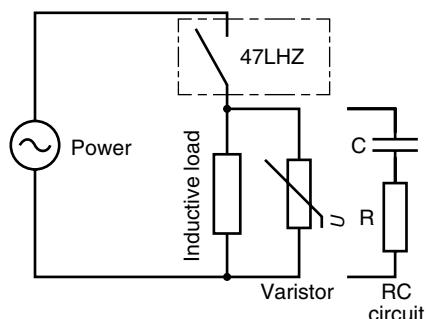
\* It is effective to connect a varistor across a load with the supply voltage 24 to 28 V, and across a contact with 100 to 200 V.
