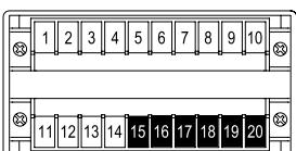
Two or four alarm contacts are output depending on the specified alarm output code.
