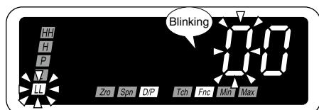
**4** Press Shift and Up buttons to set the LL (L, H or HH) ON delay time.
