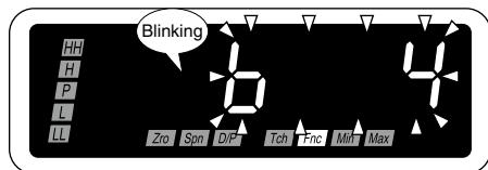
**4** Press Alarm/↓ or Scale/↑ button to apply the new setting.
