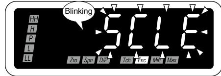
**4** Press Alarm/\downarrow or Scale/\uparrow button to apply the new setting.
