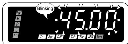
3 Hold down Alarm/↓ or Scale/↑ button for 1 second or more to return to Measuring Mode.
