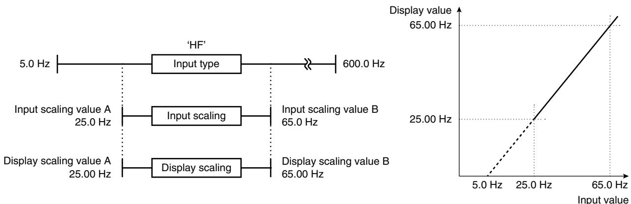
Input type: type of input signal to 47LHZ (measuring range)
